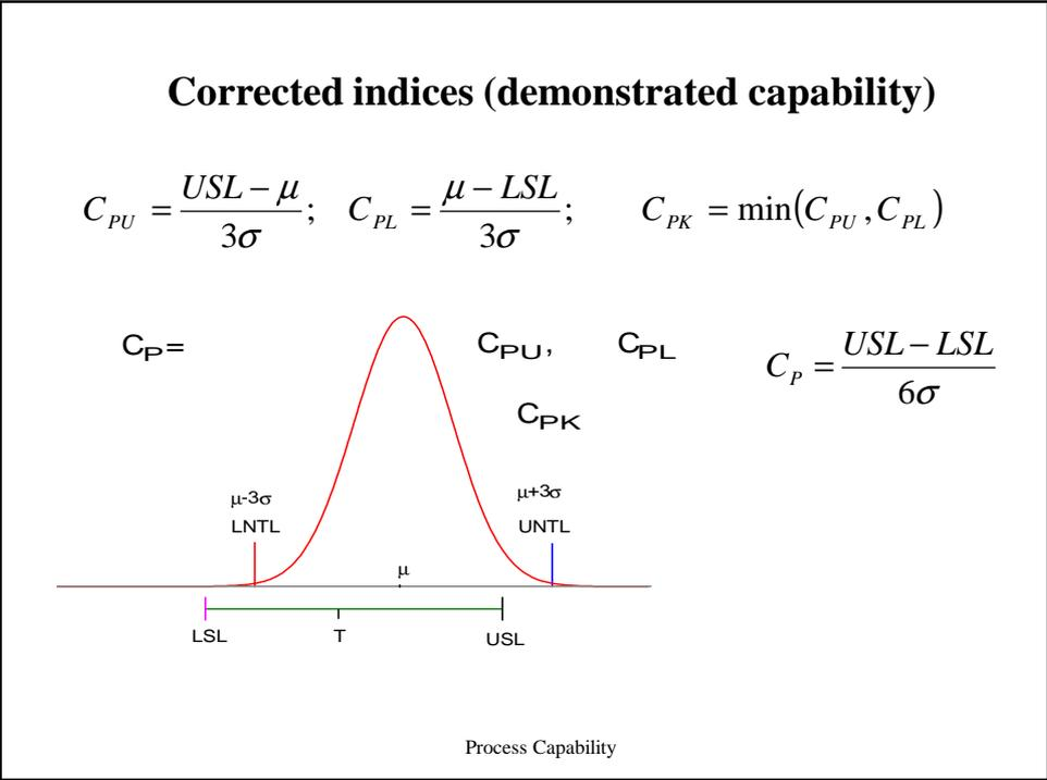
$$C_{PU} = \frac{USL - \mu}{3\sigma}; \quad C_{PL} = \frac{\mu - LSL}{3\sigma}; \quad C_{PK} = \min(C_{PU}, C_{PL})$$
