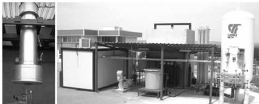
Figure 9. SCWO reactor and pilot demonstration plant of the High Pressure Process Group of the University of Valladolid (Spain)
