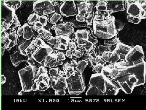
Scanning electron microscopic view of CLEC laccase Surface area (m 2 /g) 2.456
