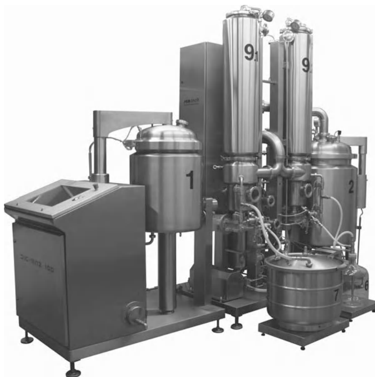
Figure 13.5 DIG-MAZ batch extractor unit. Reprinted with permission from © B. Wolfsbauer, samtech Extraktlonstechnik GmbH
