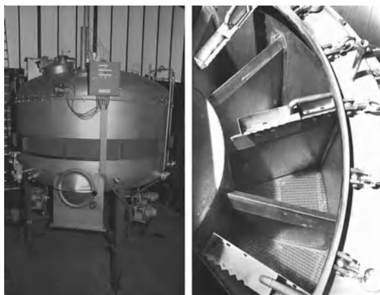
Figure 13.8 Rotary extractor (left), solid chamber (right). Reproduced by permission of PruessAnlagentechnik GmbH
