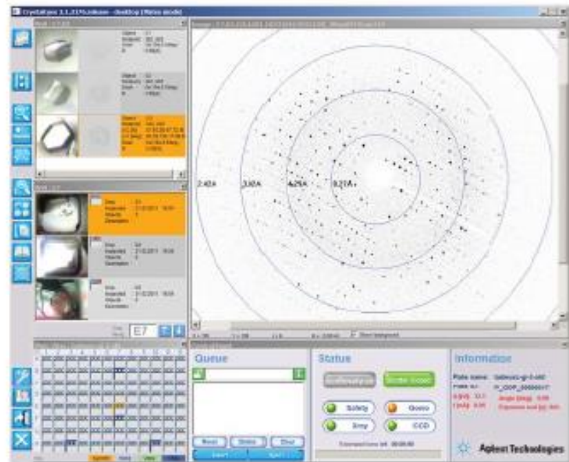
CrystalEyes with the observed diffraction image.
