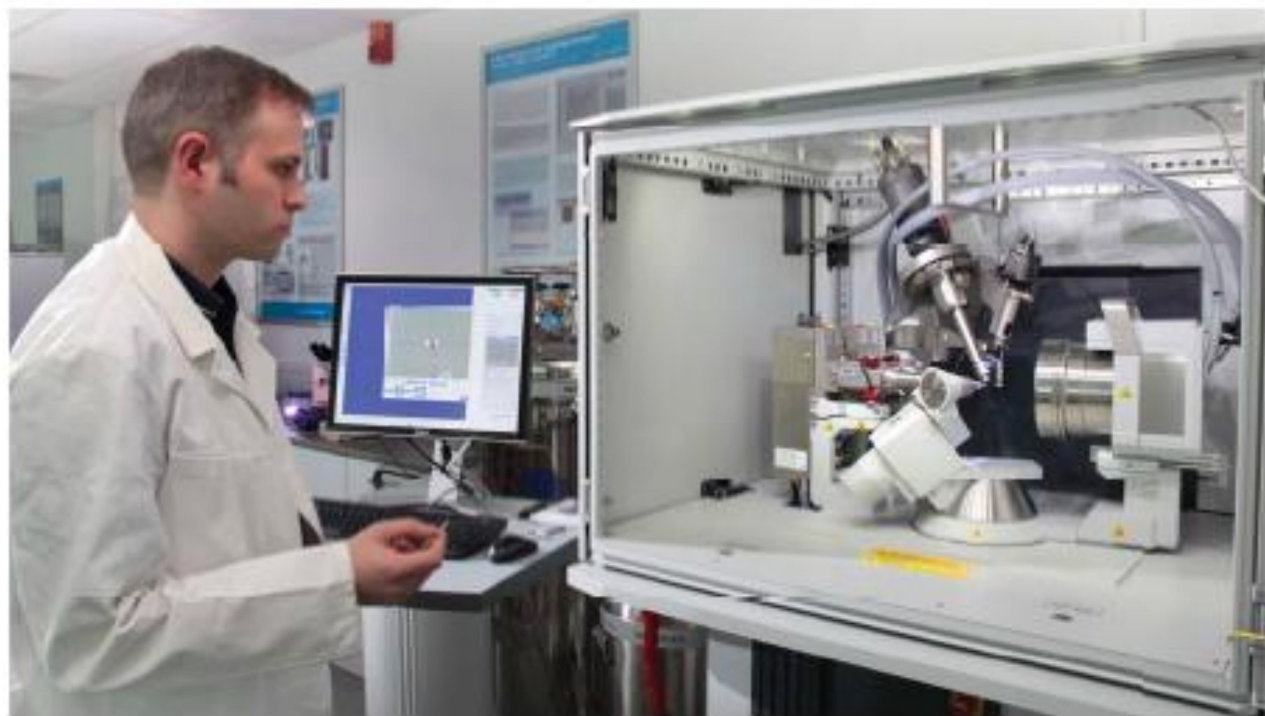
Mounting a crystal on the SuperNova.
